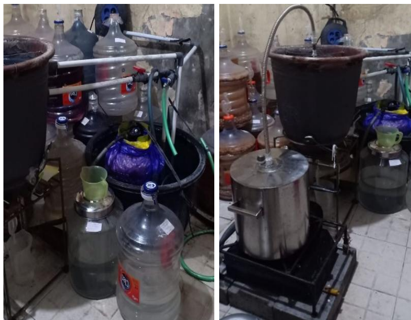
Gambar 4. Alat Distilasi Konvensional Manual UMKM Fruythatop
