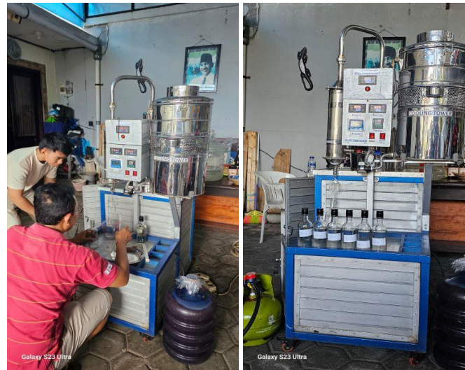
Gambar 5. Penerapan Alat Distilasi Berbasis Thermo Kontrol di UMKM Frythatop
