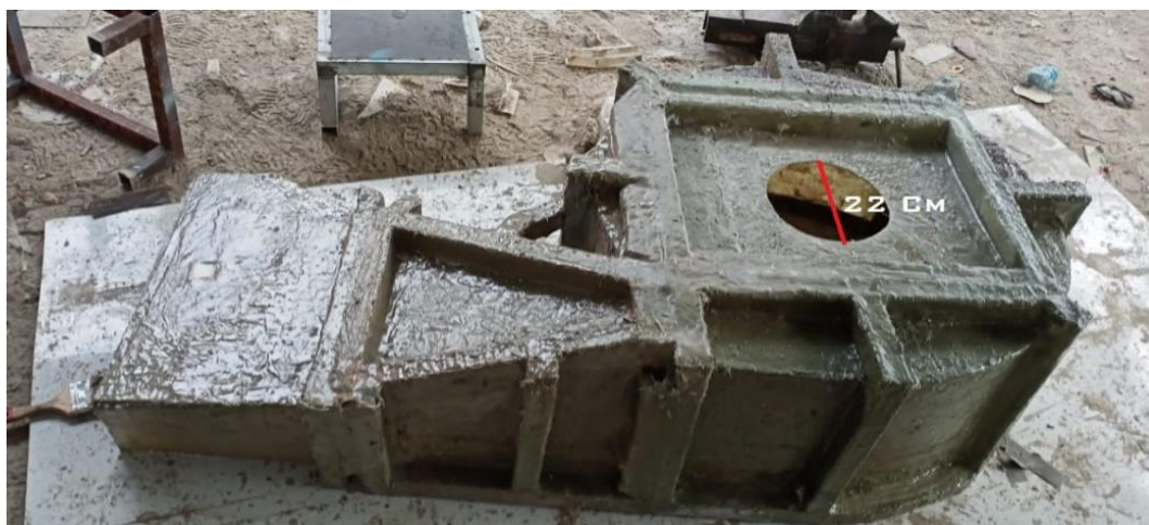
Gambar 5. Hydro Vortex System Chamber (Outlet)
